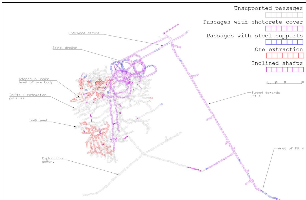
Figure 4.3 – Geotechnical plan of the Gadir underground mine (current at time of report)
